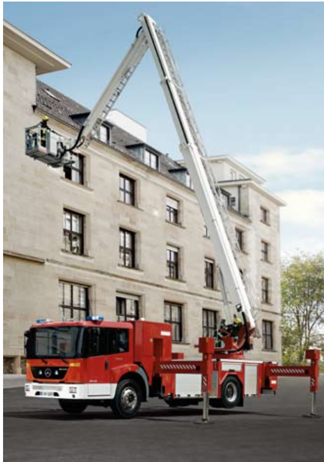
Scaling new heights: once the Econic has been correctly positioned, the stabiliser arms in combination with its excellent weight distribution ensure optimum stability as well as maximum reach and flexibility
