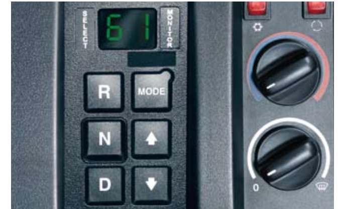
Effortless gear changes: the gearshift buttons for the standard 6-speed automatic transmission with hydraulic torque converter
