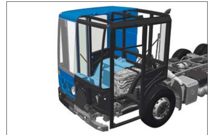
Lightweight and safe: the lightweight-aluminium Econic cabs are fully crash-tested and meet the requirements of the European crash-test standard ECE R29/2
